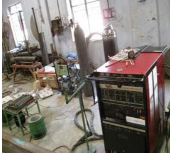
Fig 2.3. Lincoln Electrical square wave TIG 355 GTAW machine
