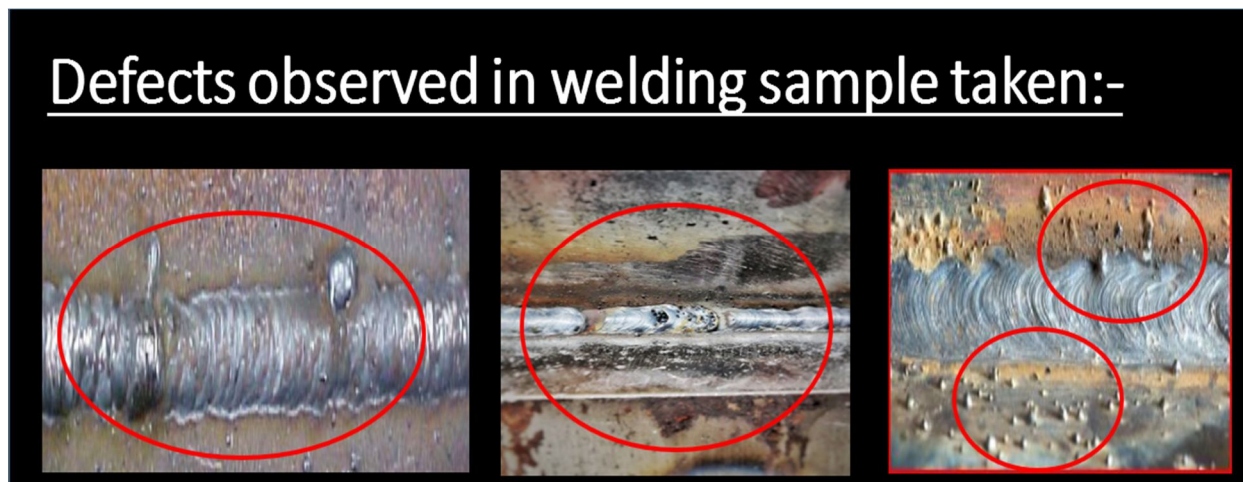
Figure 4 – Defects Observed in Rejected Welding Samples (S1) Taken (without paint)
