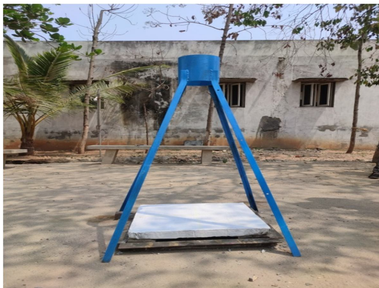
Fig.2: Self-Fabricated Impact Instrument
