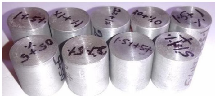
Fig. 6 Hardness Test Specimens(Before testing)
