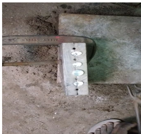
Fig. 5 Casted specimen in the die
