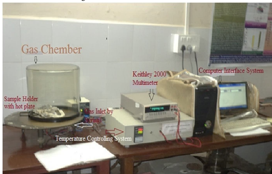
Fig. 3 Gas sensing setup used in present work
