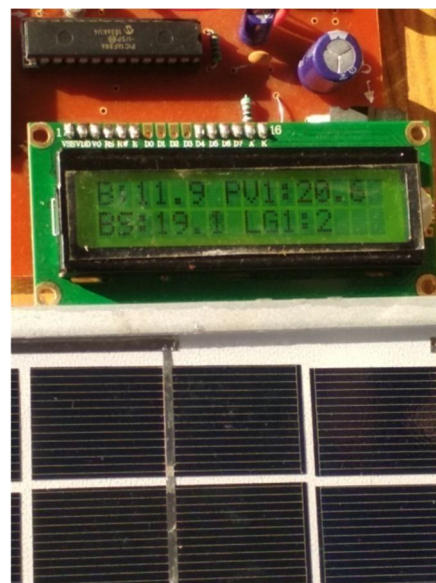
Fig.5 Panel and Battery Result on LCD
