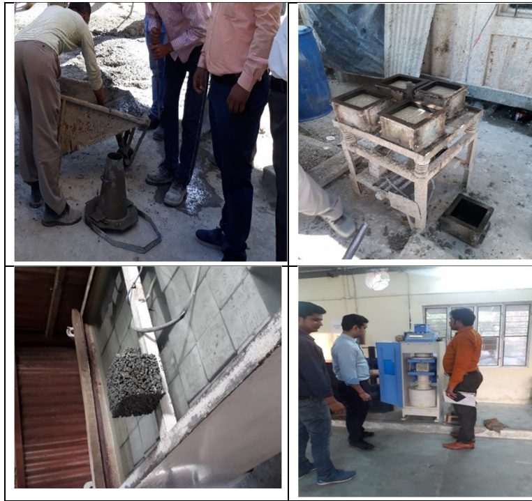
Figure 3: Preparation, curing and testing of concrete cubes adopted from project site
