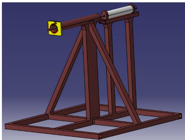
Fig.B CATIA Model Of Knotting Mechanism
