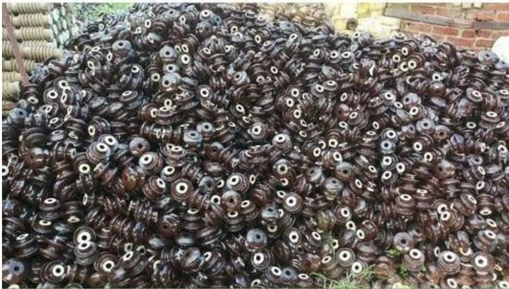
Fig.1 Ceramic Electric Insulator Waste
