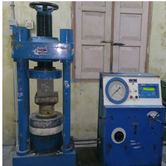
Fig.3 Compression test on concrete cubes
