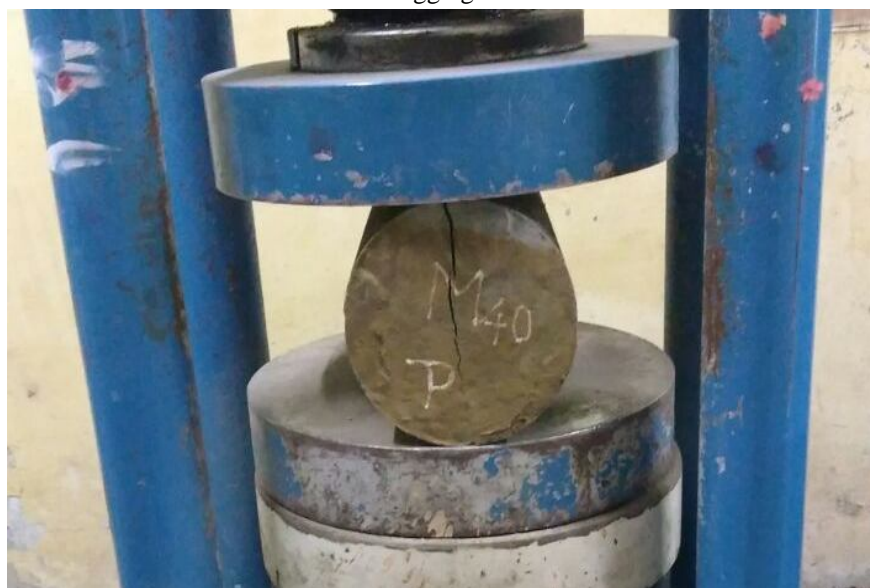
Fig.6 Failure of cylindrical specimen
