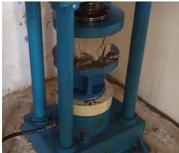
Fig.5 Failure of cube specimen
