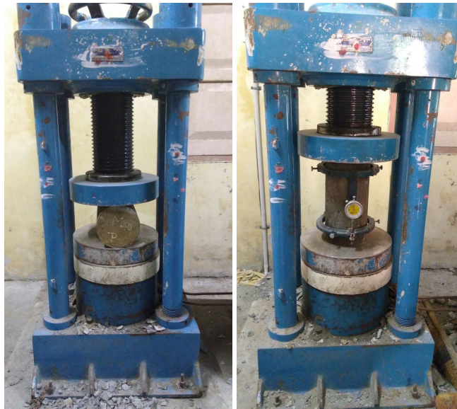
Fig.4 (a) Test setup for splitting tensile test (b) Test setup of E for concrete
