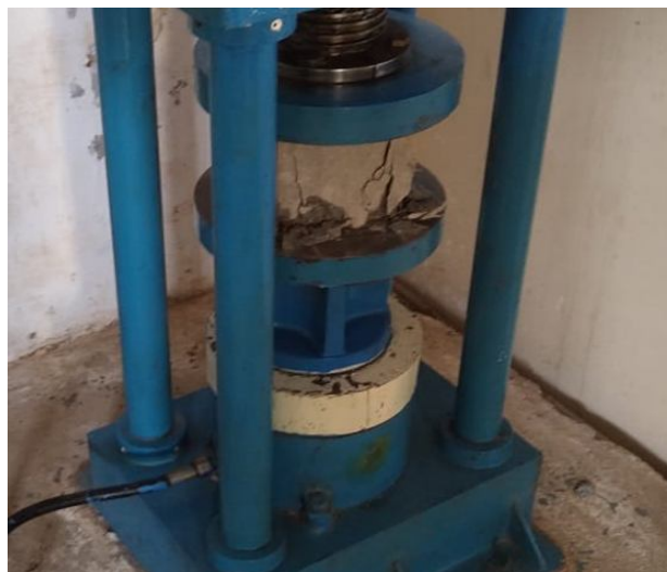
Fig.5 Failure of cube specimen
