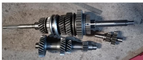
FIG. 3 Main shaft & reverse shaft with gears
