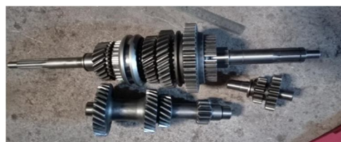
FIG. 3 Main shaft & reverse shaft with gears
