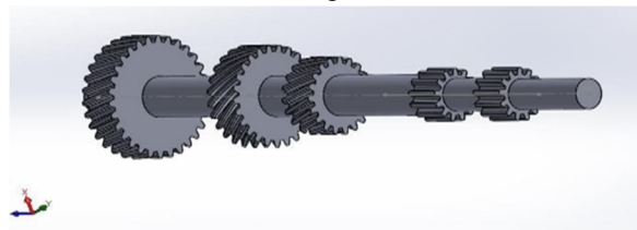
Fig. 7 CAD Design of REVERSE SHAFT
