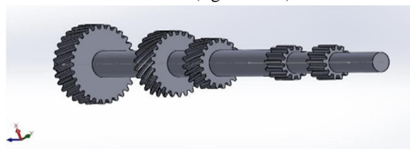
Fig. 7 CAD Design of REVERSE SHAFT
