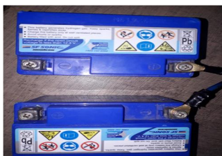
Fig 2: Lead acid battery
