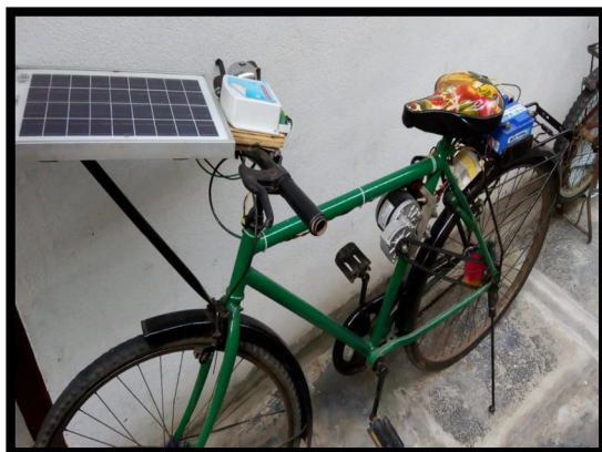
Fig 13: Fabricated model of E- bicycle
