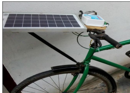
Fig 11: Solar panel & controller fixation
