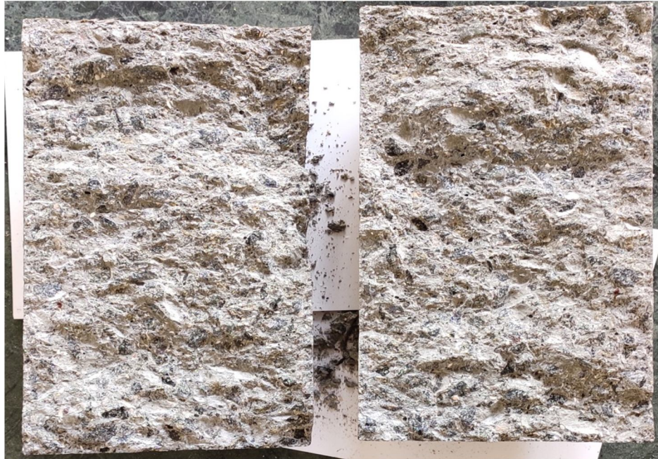
Fig.5: Failure pattern of specimen
