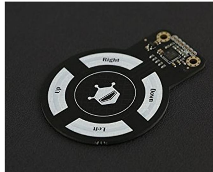
Figure 2 DFRobot 3D gesture sensor
