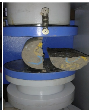
Fig 3: Split Tensile Strength Test
