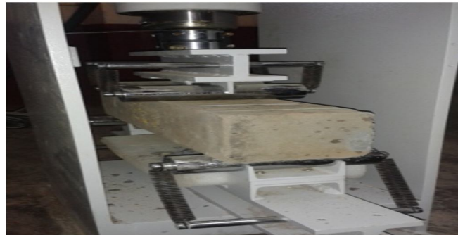
Fig 4 Flexural strength Test
