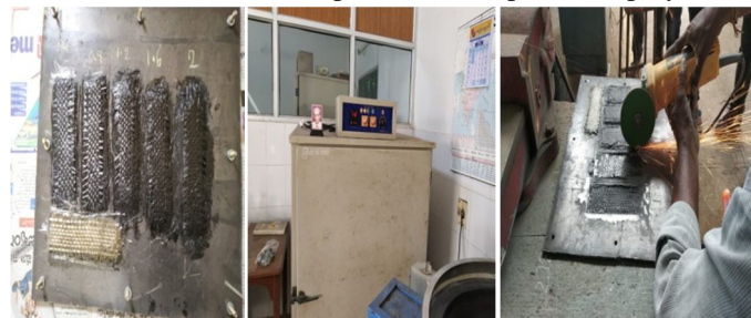
Fig. 2 Fabrication process of E-glass/epoxy/MWCNT laminates
