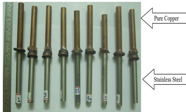
Figure 2. Specimens after friction welding process
