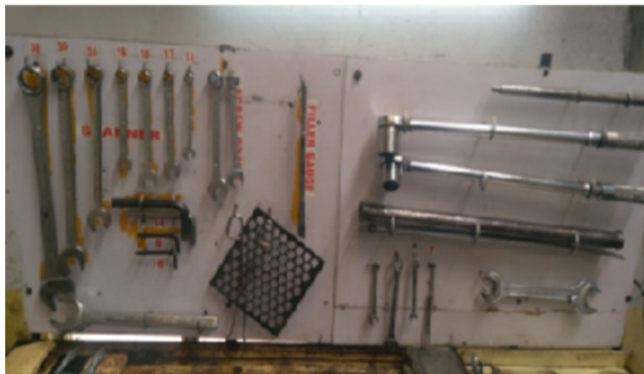
Fig.1 Poka yoke of spanner board
