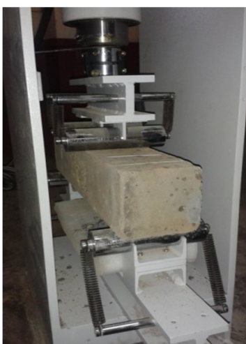
Fig 4: Flexural Strength Test
