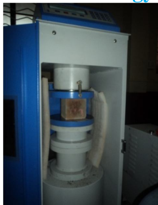
Fig 2: Compressive strength Test
