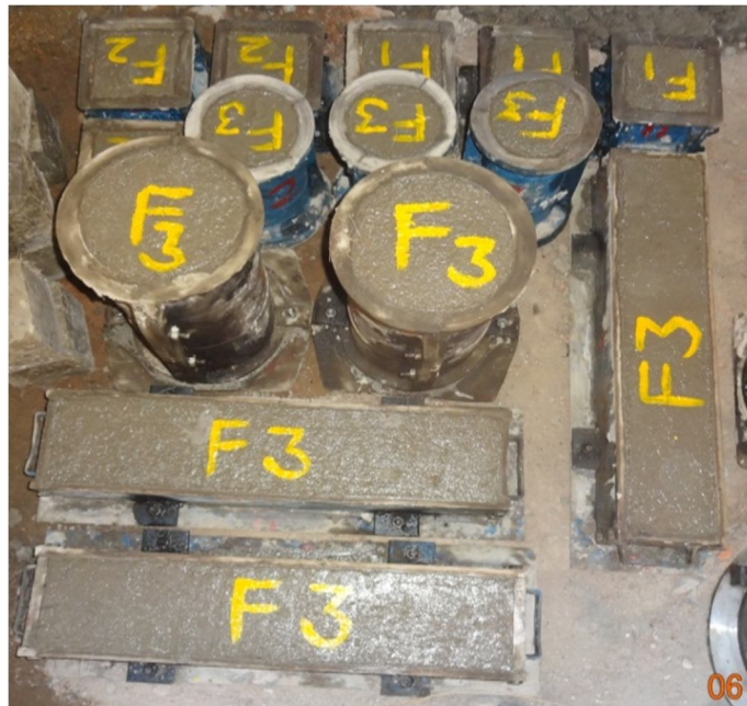
Fig 1: Casting of specimen
