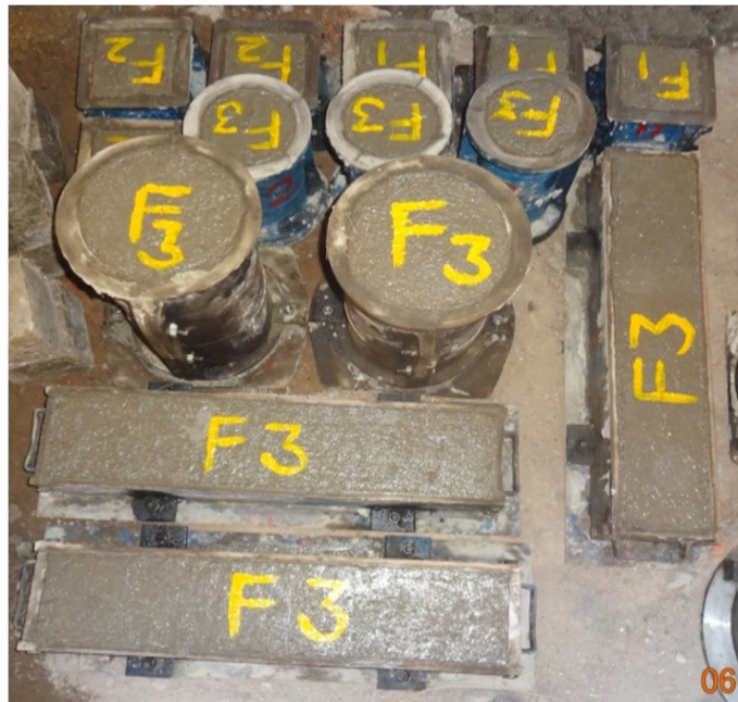
Fig 1: Casting of specimen
