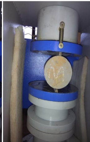
Fig 3: Split Tensile Strength Test
