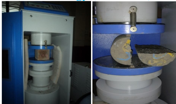
Fig 2 & 3: Setup for compressive and split tensile strength.
