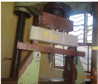
Fig 4: Setup for Flexural Strength Test
