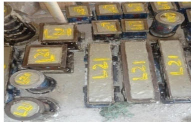
Fig 1: Concrete placed in moulds
