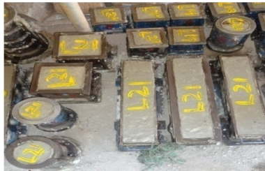
Fig 1: Concrete placed in moulds
