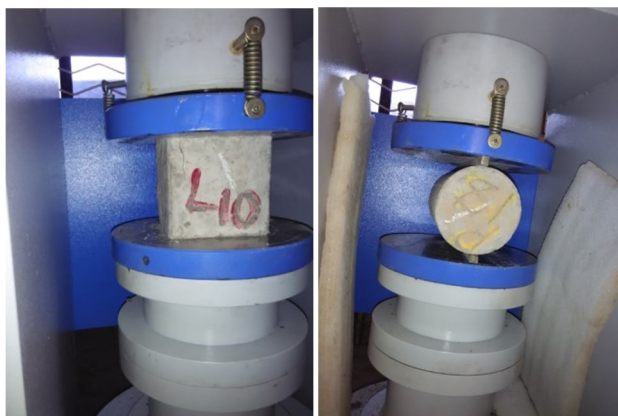
Fig 2: Compressive Strength Test Fig 3: Tensile Strength Test
