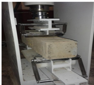
Fig 4: Flexural Strength Test
