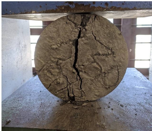
Fig.2. Split tensile strength testing
