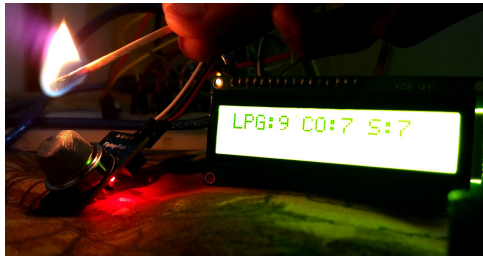
Fig. 5 LCD displaying concentration of gases.
