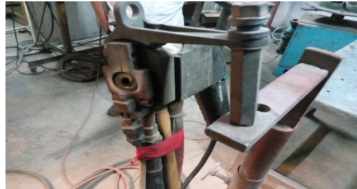
Figure 1.4.1. Plasma spray coating gun.
