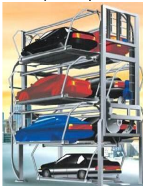
Figure 7 Rotary parking system parking assembly [15]
