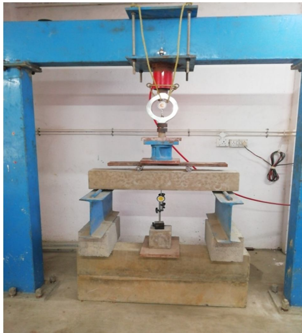
Figure 2 Testing of beam
