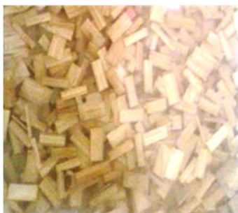
Fig.1. fabricated short bamboo fiber reinforced composite.
