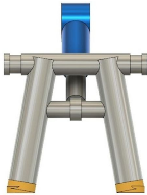
Fig. 4 (a) Front View of automatic centre stand when first Hydraulic Cylinder operated
