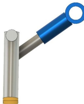
Fig. 3 (b) Side View of automatic centre stand when first Hydraulic Cylinder operated.
