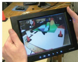
A handheld AR system displaying a three dimensional graph registered to the cones and table. (CSM, 2011)
