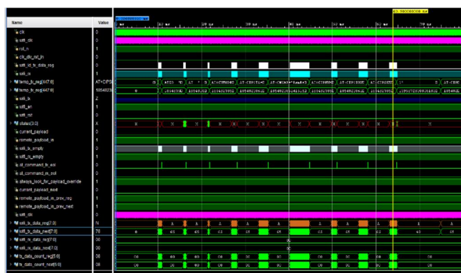
Fig 9. Wi-Fi module interface with FPGA
