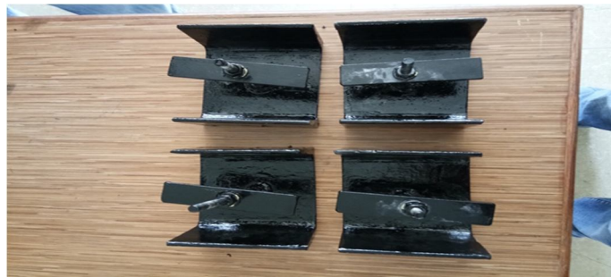
Fig. No.3.19 c-channel fabrication
