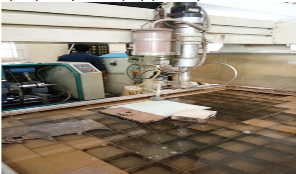
Fig. No.3.18 water jet cutting
