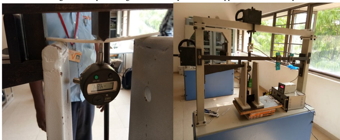
Fig. No.4.3 dial gauge and deflection test
