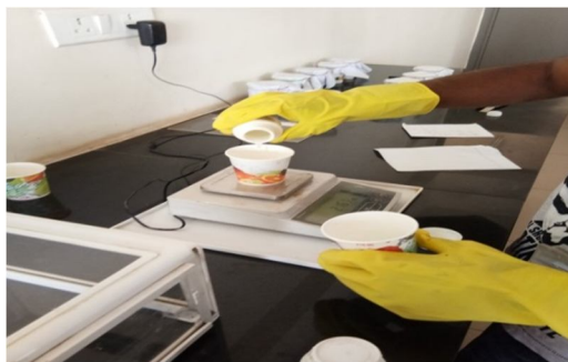
Fig. No.3.9 epoxy ly556 and hardener-hy951 preparation
