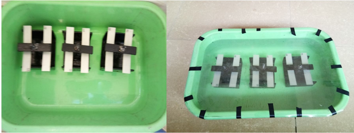
Fig. No.4.4 specimen submerged in sea water
