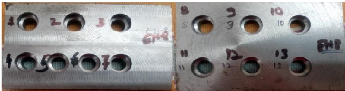
Fig-4.0.3:- EN8 work piece material with contour holes
