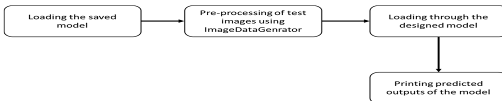
Fig 3: Methodology of Testing the Model
