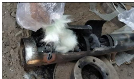
Figure No 12 - Fill the charcoal and glass wool
