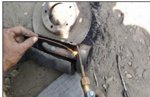
Figure No 10 - Insert recirculating pipe
