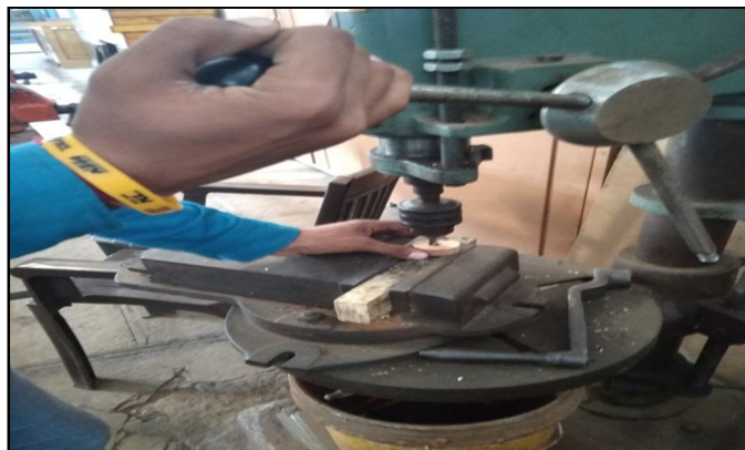
Figure 10. - Drilling procedure of Crankshaft
