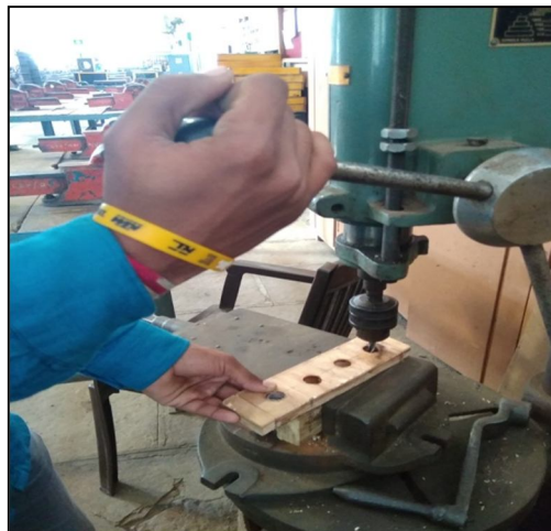
Figure 8. - Drilling Procedure of mounting
