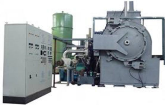
Fig 3.1.2 Heat treatment of specimens on Quenching oil furnace
