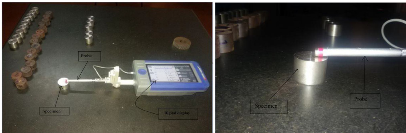
Fig 3.1.4.1 Surtronic 3+ tester measuring surface roughness of specimen
