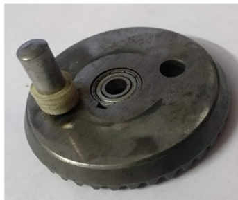
Figure 5: Spiral Bevel Spur Gear With offset pin
