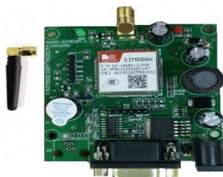
Fig 5: GSM 900A module of our system
