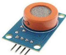
Fig 4: MQ3 Alcohol sensor of our system
