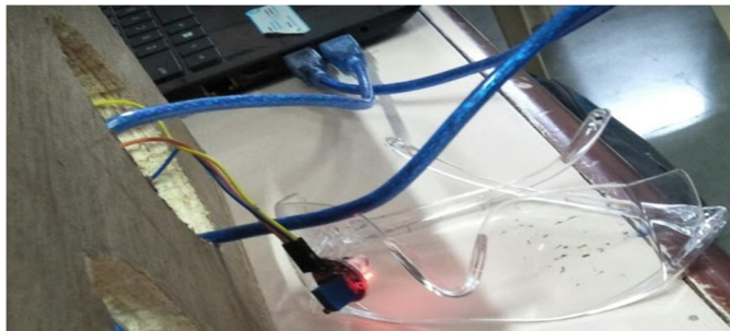
Fig 3: Eyeblink sensor module of our system
