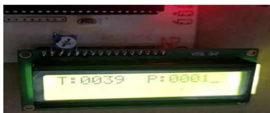
Figure 7: Showing Temperature and Pressure values on LCD
