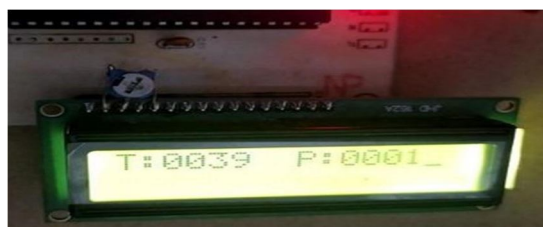
Figure 7: Showing Temperature and Pressure values on LCD
