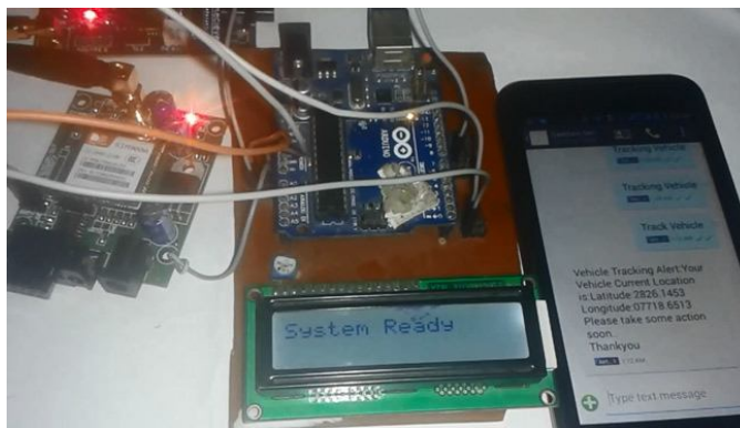
Fig 7: Messaging Facility In system
