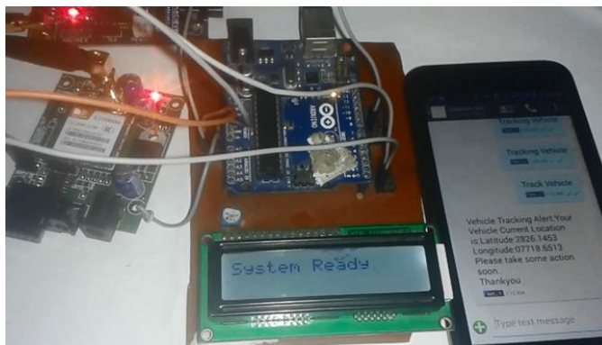
Fig 7: Messaging Facility In system
