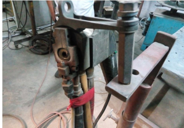
Figure 1.1. Plasma spray coating gun.
