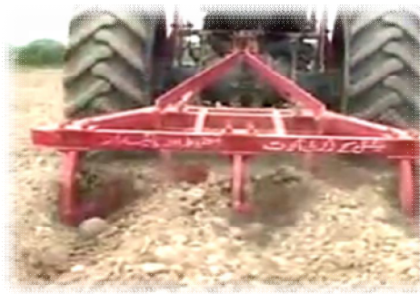
Fig: 1(c) Ploughing action Raja MB Plough in Experimental field Plot
