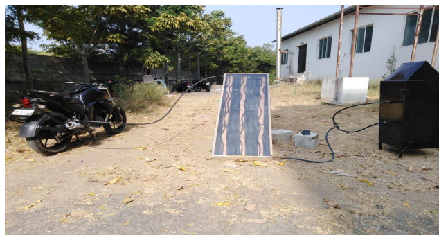
Figure 3.2 Experimental setup by bike exhaust as inlet
