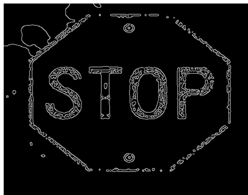
Fig4. (c). Canny detected Image with framework of Gaussian, median and Wiener filter
