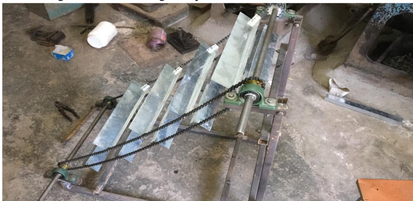
Fig. 1 Our Model River Cleaning Machine
