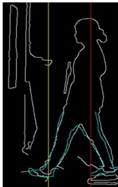
Figure6: Top head center line is represented by red line and average leg template distance is represented by yellow lines.
