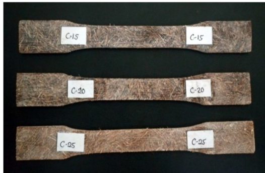
Fig.11(a). Coir fiber composite tensile test specimens before testing
