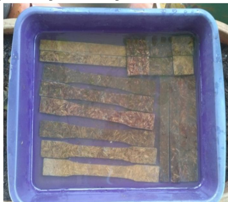
Fig.13(b). Specimens in rain water after 15 days
