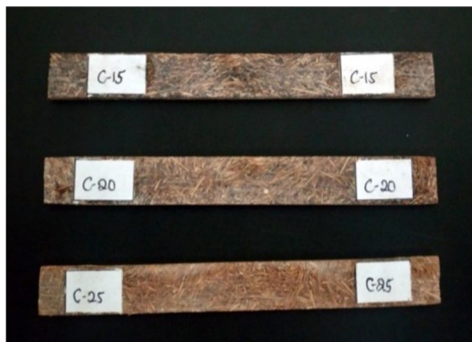
Fig.12(a). Coir fiber composite bending test specimens before testing
