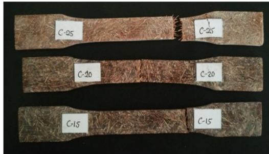
Fig.11(b). Coir fiber composite tensile test specimens after testing
