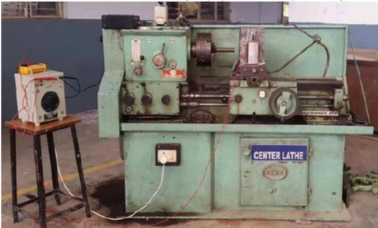
Figure 2 Centre lathe with MAF setup
