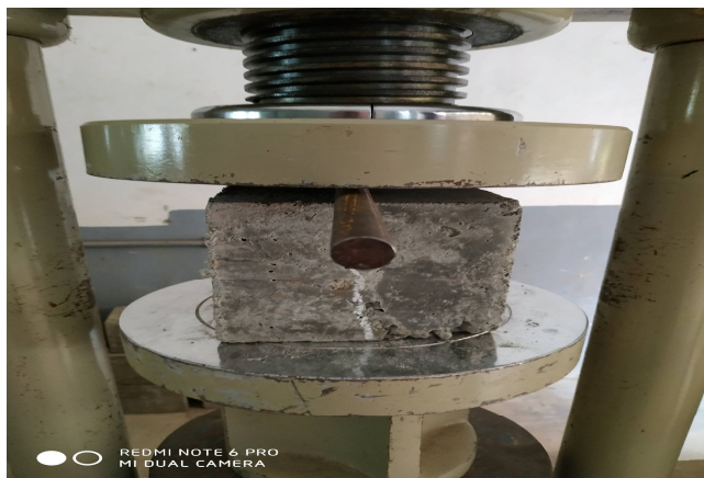
Fig.14 Tensile bond strength on cube
