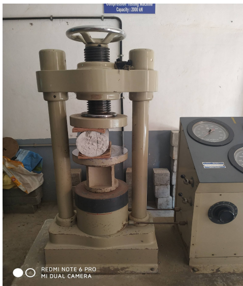
Fig.12 Split Tensile Test on cylinders
