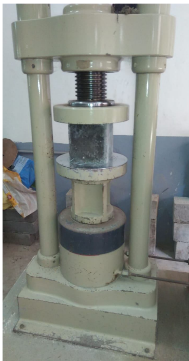
Fig.13 Compression test on cube
